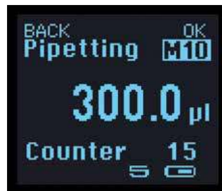
M10 indicates that 300 µl pipetting has been saved in memory place 10.
